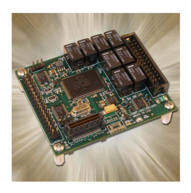
ACCES I/O Products' Pico-I/O Module Provides 16 TTL/LVTTL Digital I/O and 8 Relay Outputs
